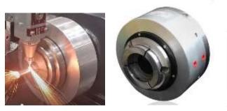
It adopts pneumatic clamp design and it can modulate the center of the materials for pipes automatically and precisely. The diagonal adjustable range is 16-60mm.
