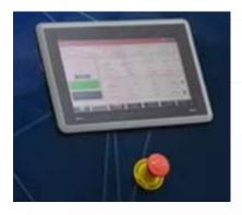
User Friendly 10" Industrial touch screen control panel with emergency button. Inside the electrical panel, all servo drivers are connected to the PLC, so it is easy to control servo drivers directly from the screen.
